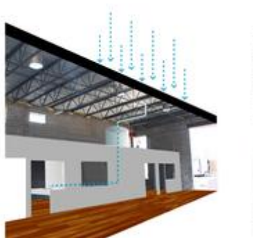
Rainwater Collection System Diagram - Photo Credit: Julie
